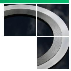
Camprofile gaskets consist of a serrated metallic core, provided with or without support rings. These are generally provided with a soft facing made from graphite, PTFE or high temperature mica material.
